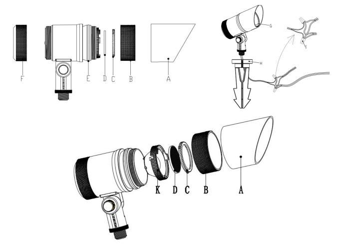
A - Shroud B - Front Cover Lens C- Lens Accessory Lock Ring D -Hexagon Louver E -Fixture Body F -back cover G- Assembled Fixture H-Spike I-Waterproof Wire Nuts
