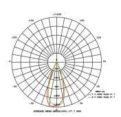
Construction: Brass Finish: Antique Brush Lead Wire: 6ft long Mounting: LAP-002 Wattage: 5W or 10W Operating Voltage: 10-15V Lumens: 375LM or 600LM Beam Spread: 15°, 38°, 60°
