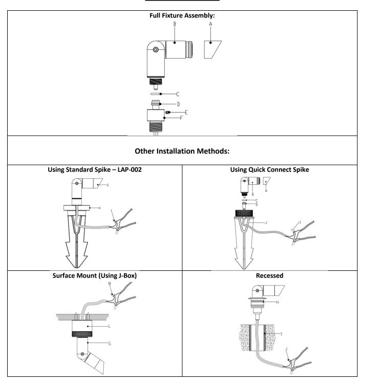
A - Shroud B – Module/Knuckle C- O-Ring D - Female Connector E- Set Screw F-Lock Nut J- Spike I-Waterproof Wire Nuts
