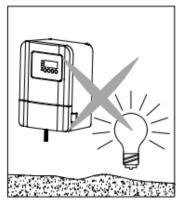
1.4 Only applies in AUTO MODE. Photocell will not operate properly if installed too close to nighttime light source.
