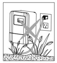
1.1.Outdoor use, weather proof. 1.2 Mount the transformer 1.3 Only applies in AUTO MODE. Do not install behind shrubs. It will affect photocell for Auto dusk-to-dawn mode.
