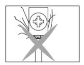
2.4 Verify that there are no loose cable strands. 2.5Replace the bottom plate and close the front
